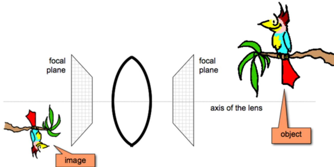
Lenses actually have **two** focal planes, symmetrically placed, one on each side.
