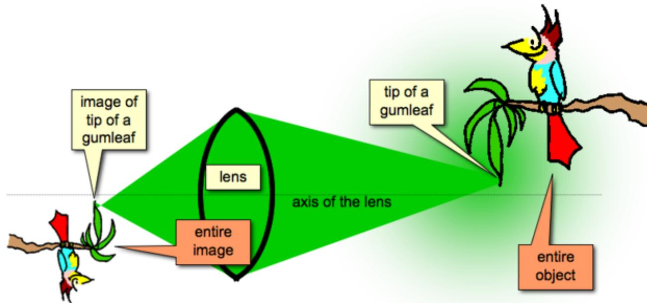
The lens bends the light, and focuses it in a small [area](#). This happens for the whole object, and a complete image forms.
