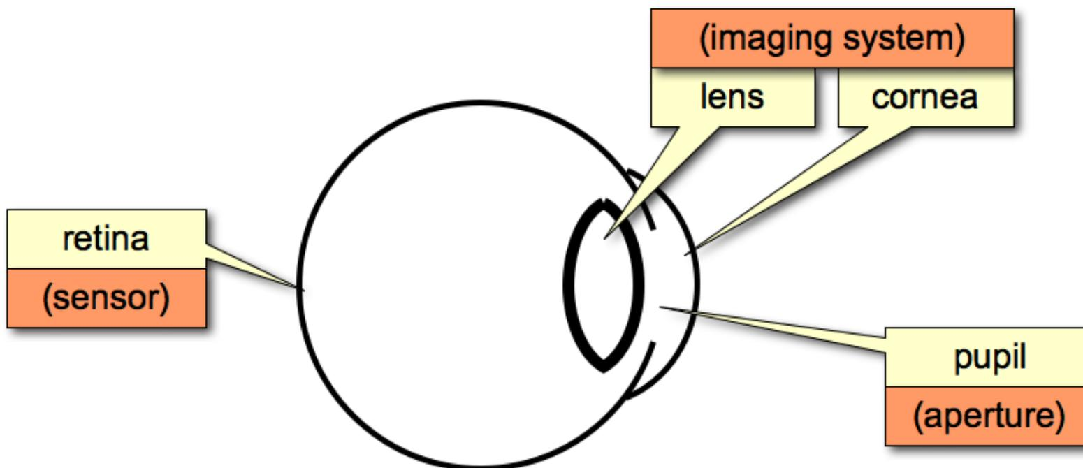
First of all, we have to understand the imaging system, and that means understanding how convex **lenses** collect light and form images.
