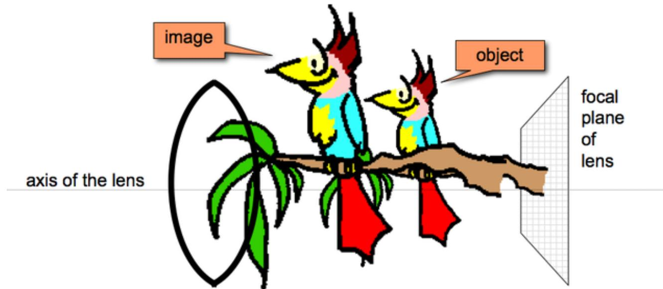
If the object is between the **focal plane** and the lens, then the image is large and near the object . This is how a **magnifying glass** works.
